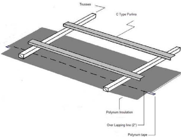
Guide for overlapping joints into wooden trusses:
